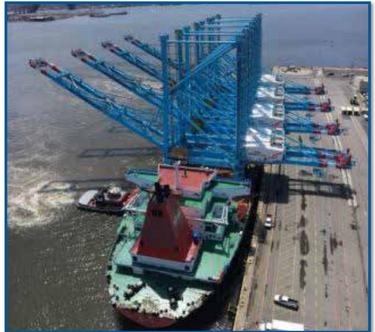
*The four gantry cranes are designed for operations on today's largest container vessels*
