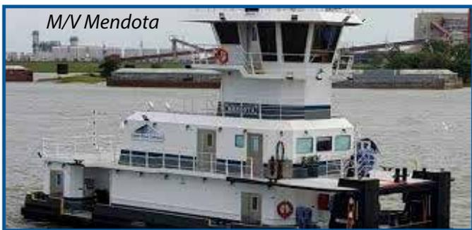
It took less than six months for C&C Marine and Repair based in Belle Chasse, Louisiana, a Signal Member since 2016, to complete the 2,013 hp triple-screw towboat *M/V Mendota*, the first new construction vessel ever to join the fleet of Upper River Services, LLC, St. Paul, Minneapolis.
